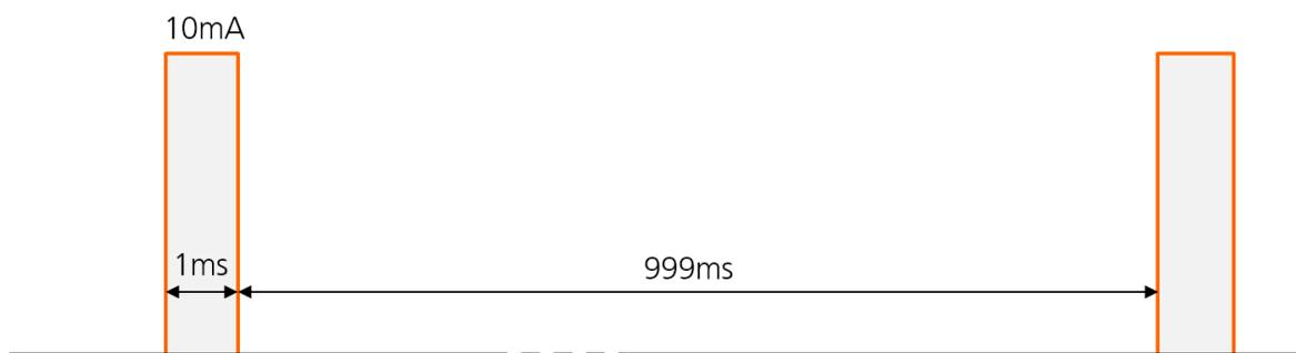
Figure 4 - Typical current profile of a BLE device
