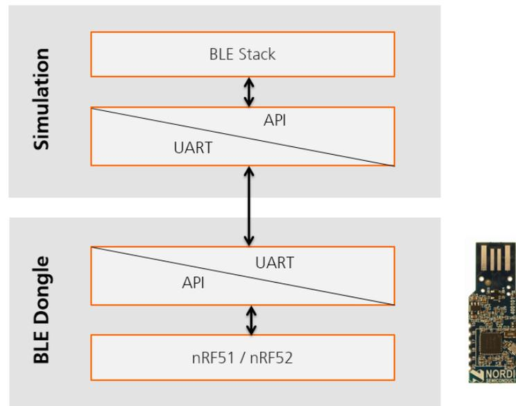
Figure 3 - BLE Support in simulated devices
