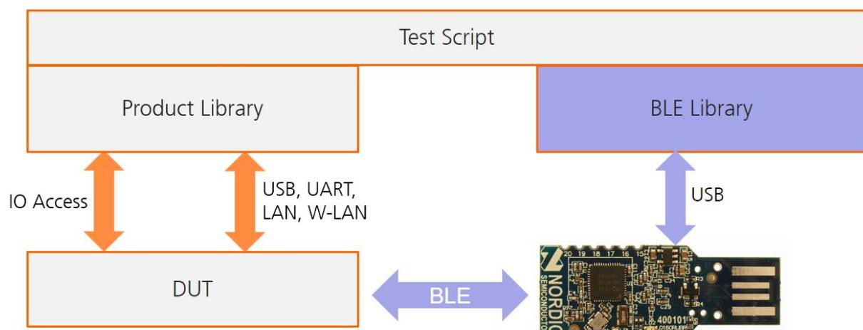
Figure 7 - System-Test setup for BLE tests
